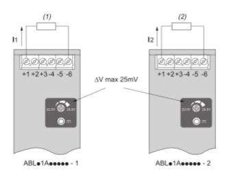
(1):  $R_{Load1}$ (2):  $R_{Load2}$  $R_{Load1} = R_{Load2}$  $I_1 = I_2 = -I_{nom}$
